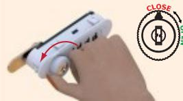
1. TURN THE DIALS TO THE SET CODE, E.G. 1-1-1-1 AND ROTATE THE KNOB TO CLOSE POSITION.
