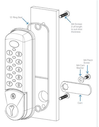
Holes A & B diameter 4.5 / 5.0mm Hole C diameter 17.0 / 17.5mm Recommended screw fixing torque 0.5Nm min.
